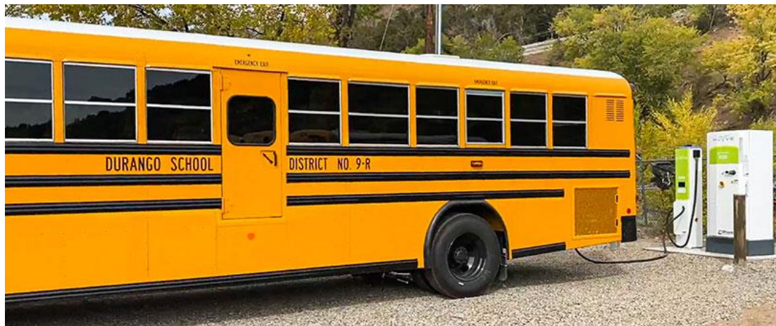
Figure 8: Blue Bird Electric School Bus Connected to Nuvve Bidirectional Charger in Durango, CO
